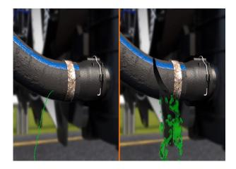
Rarely used hoses can become dry and cause external cracks.
