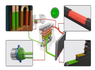
Corrosive radiator fluid can wear hoses from the inside and cause damage to the hose itself.
