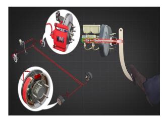
Each wheel of a car has either disc brake assembly or drum brake assembly which helps the vehicle slow down A moving vehicle has a huge amount of stored energy, so stopping the vehicle means the movement energy needs to be converted to another form. On hybrid vehicles, a lot of the movement energy is stored in the battery so that it can be reused, but on non-electric vehicles, the movement energy is converted to heat energy by the braking system. Let's take a look at how that system works.
